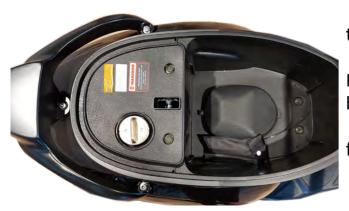
Use the switch lock to unlock the saddle to open the luggage compartment.
