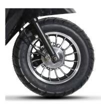
The correct tire pressure is essential for the safety and driving of the scooter. Tire pressure should be checked before each use. While driving the scooter, tire temperature and pressure will change depending on speed and load. For this reason, tire pressure should only be checked and adjusted when the tires are cold. Normal tire pressure (cold)
